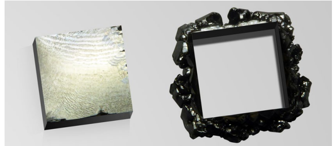
CVD block after coring process
